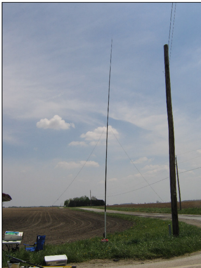
This is the vertical antenna we used. An SGC tuner is at the base and radials are spread across the grass, road and empty corn field.
