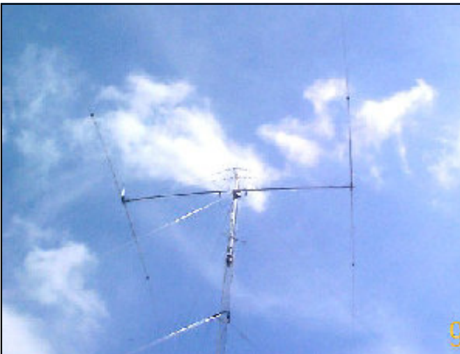
The 80 meter beam finished at 150'
